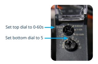
Adjust CSR113 with included adjustment tool as instructed below.
