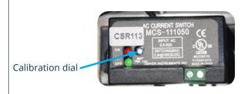
**RED LED** = Normal operation, mixer operating above set point (normal amps). **GREEN LED** = Out of water, mixer operating under set point (low amps).
