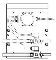
Mounting plate (non US version) with two solenoid valves P/N 11705516B, and a connection box P/N 11505748.
