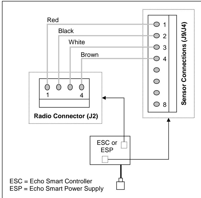
Figure 37: Connections for Wireless Radio Module (External)
