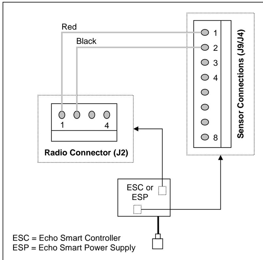
Figure 36: Connections for Wireless Radio Module (Internal)
