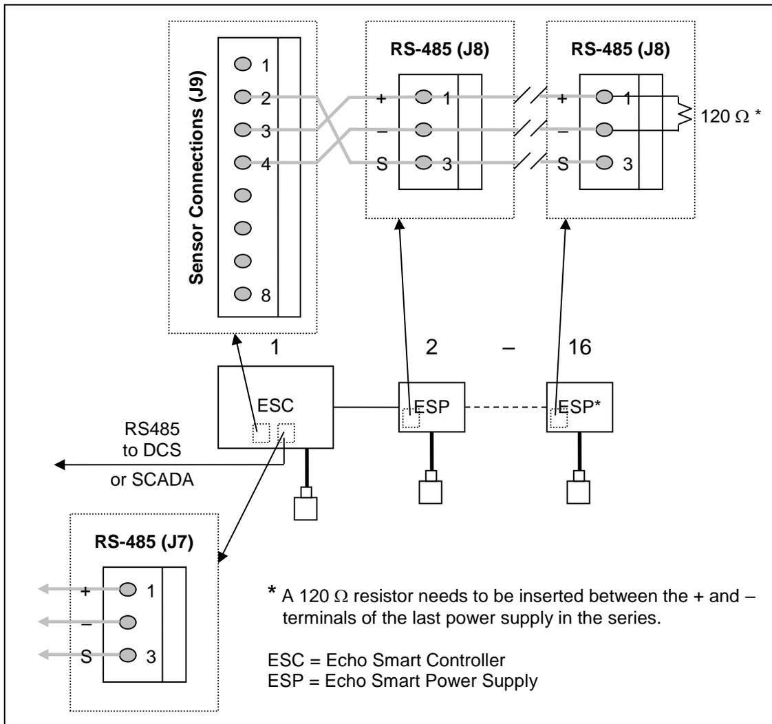
Figure 30: Single Wired Field Network
