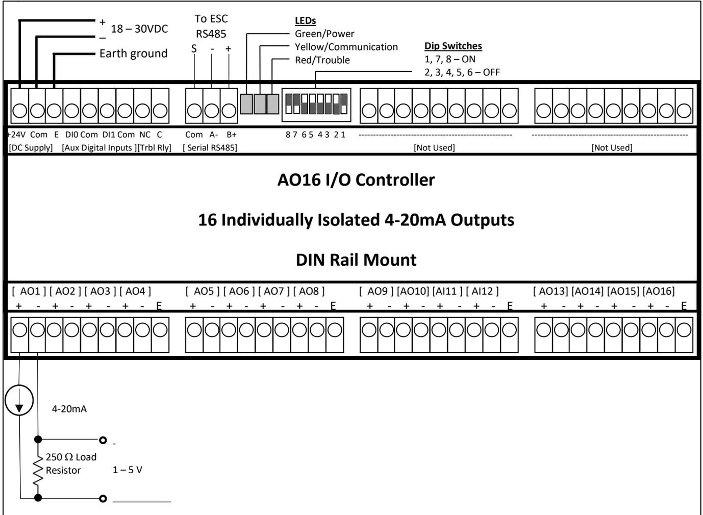
Figure 42: Analog Output Module Connections
