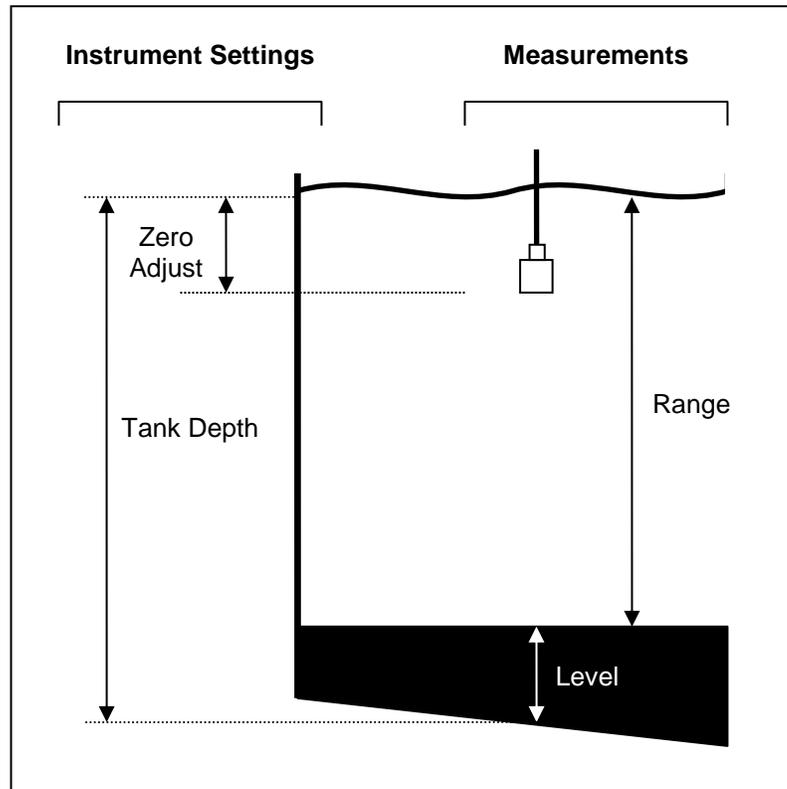
Figure 27: Tank Configuration
