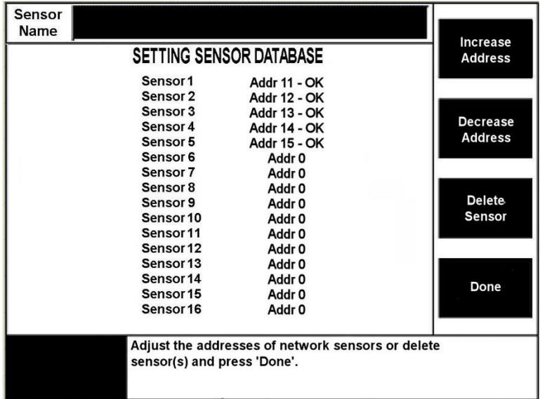
Figure 19: Modifying Sensor Database Display
