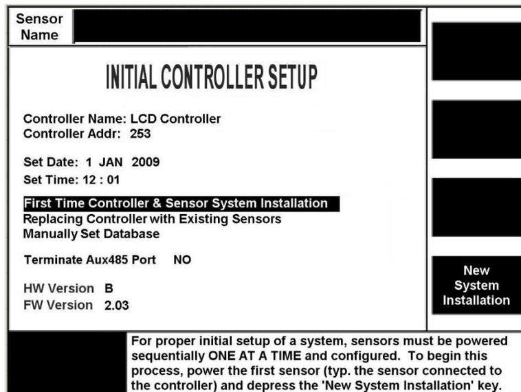
Figure 5: Initial Controller Setup
