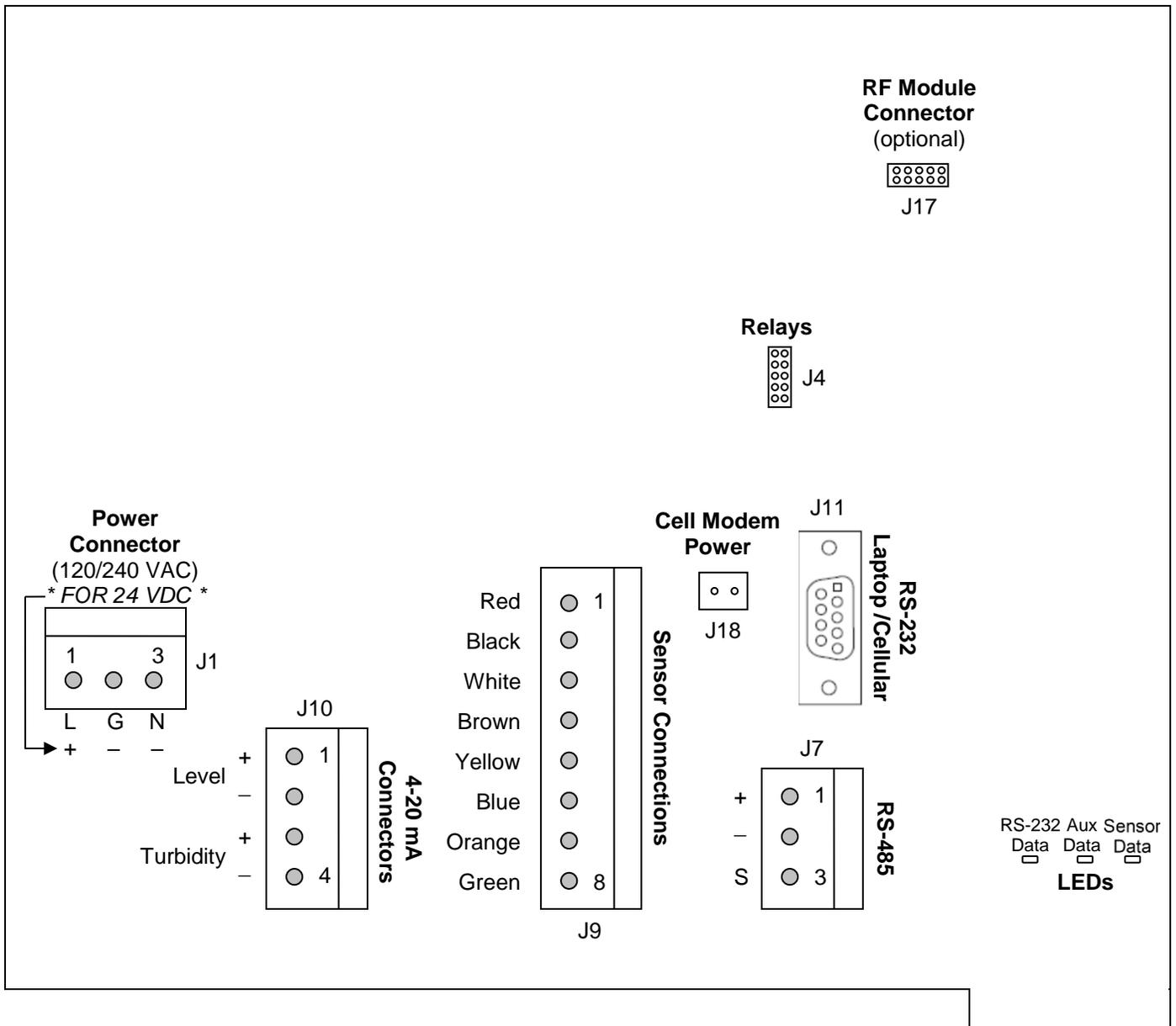
Figure 3: Connections for Controller
