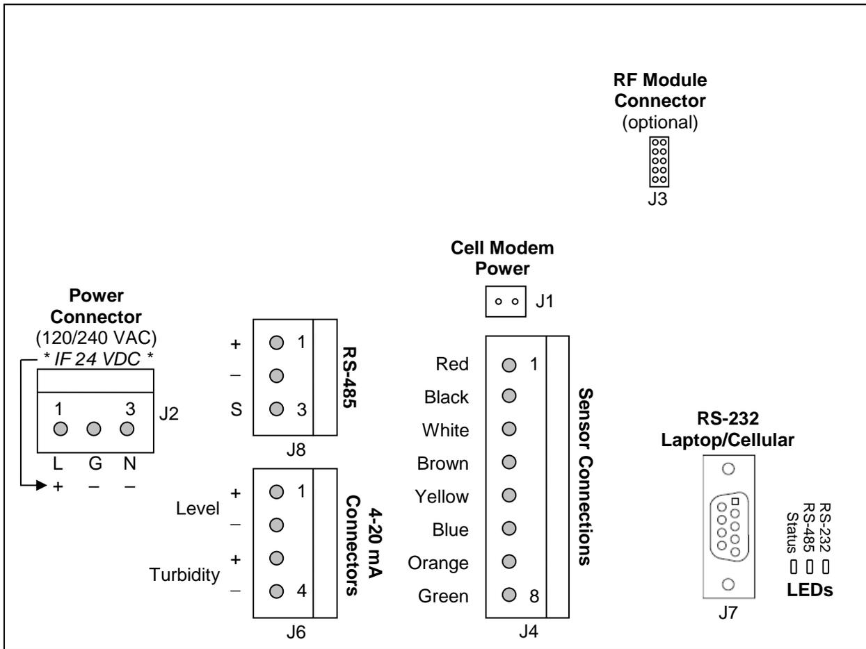
Figure 21: Connections for Power Supply
