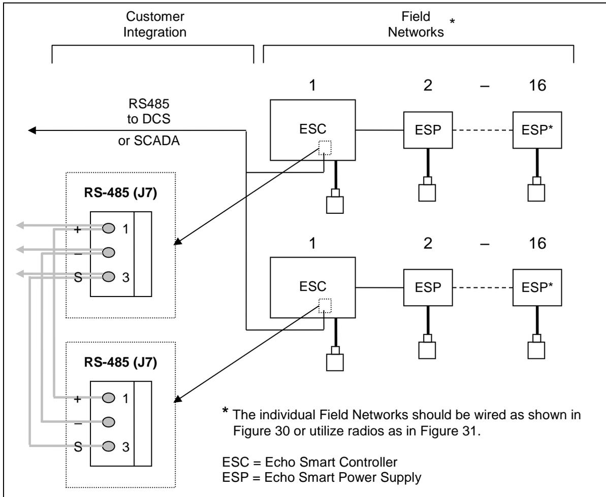
Figure 32: Integrated Wired Field Network
