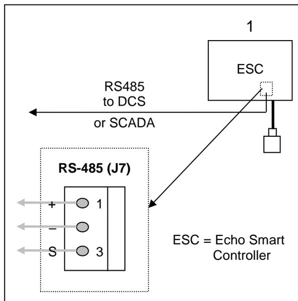
Figure 29: Controller with Single Sensor
