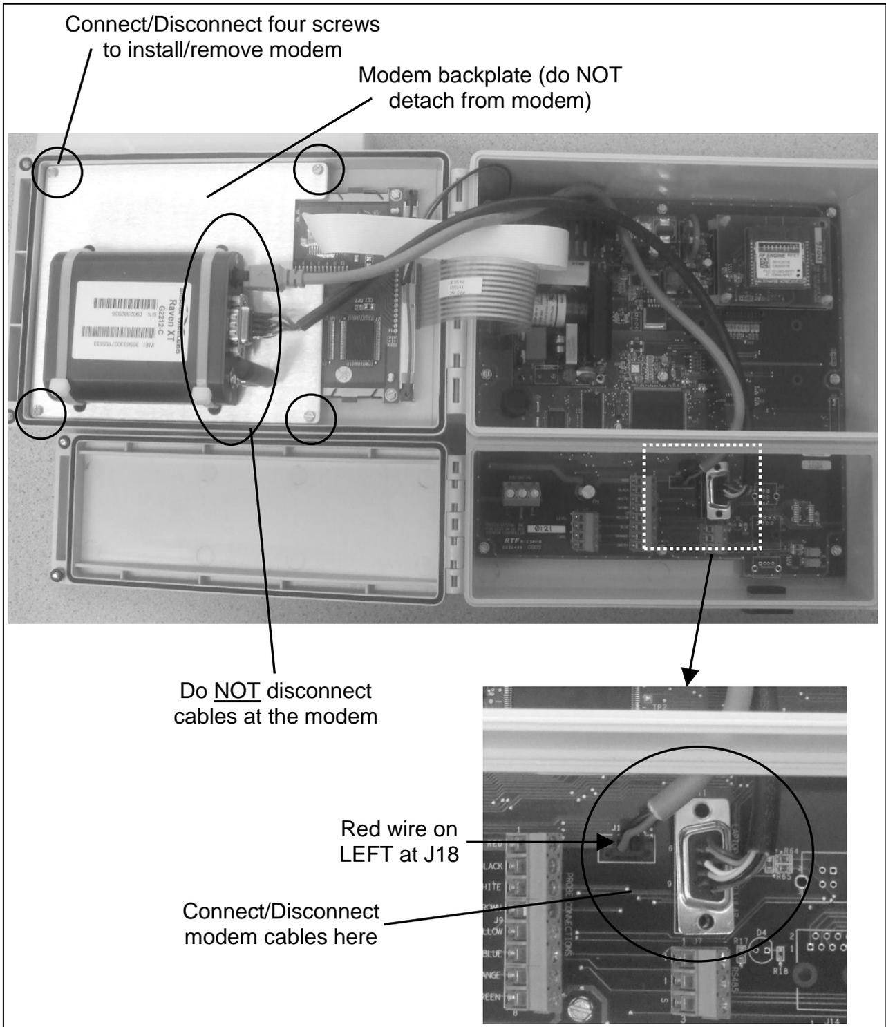
Figure 33: Proper Installation and Removal of Modem
