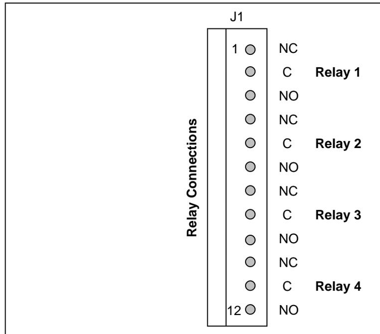
Figure 40: Connections for Relay Board
