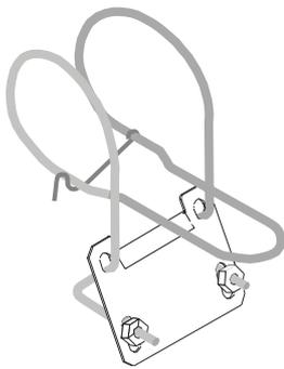
Mount the Flexible Mounting Bracket on existing handrail or on separate holder, diameter 32-50 mm (1 ¼" – 2") or square 28-42 mm (1 ⅛" – 1 ⅝"). The bent lip on the mounting plate shall be on top and faced toward the liquid or tank. Adjust the Mounting Bracket to the correct angle and tighten the nuts. The bracket shall be fixed to the rail, and must not be able to rotate around it.
