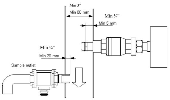
Mounting of sensor and sample outlet
