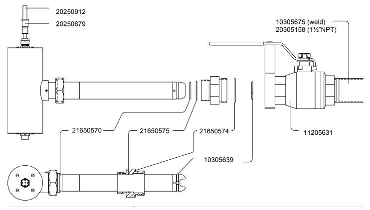
Nipple 10305675 is to be cut to make the bottom of the measure gap be at least 5 mm  $(\frac{1}{4})$  from the pipe wall.
