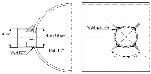
Mounting of weld end with strip iron
