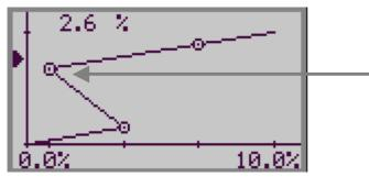
The curve goes backwards because two samples have been exchanged when entering the lab results. Higher Y-value must mean higher X-value. The curve must have a direction upwards and to the right.
