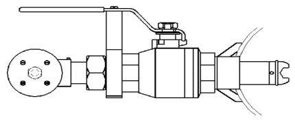
Mounting of sensor in ball valve
