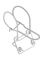
Mount the Flexible Mounting Bracket on handrail diameter of  $1\frac{1}{4}$ " -2" (32-50 mm) Ø or square  $1\frac{1}{8}$ "  $-1\frac{5}{8}$ " (28-42 mm). The bent lip on the mounting plate shall be on top and faced toward the liquid or tank. Adjust the Mounting Bracket to the correct angle and tighten the SS nuts. The bracket shall be fixed to the rail, and it shall not be able to move it.
