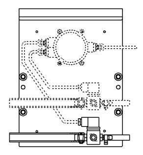
Mounting plate P/N 10305533 for one or two solenoids, outside US version P/N 11705516A (11705516 B US Version) and a connection box P/N 11505748.
