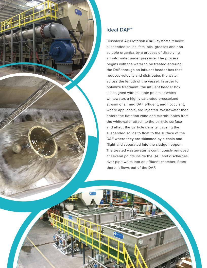
The Ideal DAF™ achieves high rate removal efficiencies at a low operational cost with a smaller footprint and longer lifespan by employing such techniques as:
