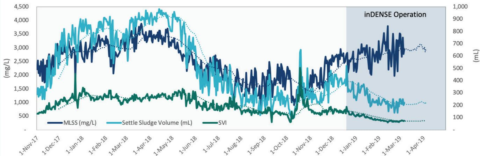
The graph above shows performance of an activated sludge system before and after installation of the inDENSE Process. Once operational, there was an immediate reduction in the Settle Sludge Volume (SSV) and sludge
