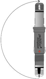
The buffer adjustment mode is initiated after app. 30 seconds - this is indicated by the LED with 3 short flashes every 5 seconds.
