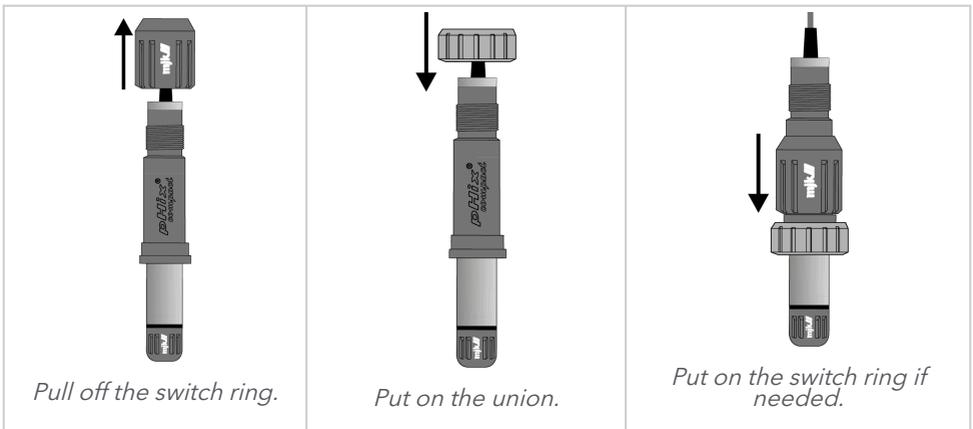
The switch ring is only used for buffer adjustment (calibration), but it is also possible to perform a [buffer adjustment](#) (see page 22) without using the switch ring.
