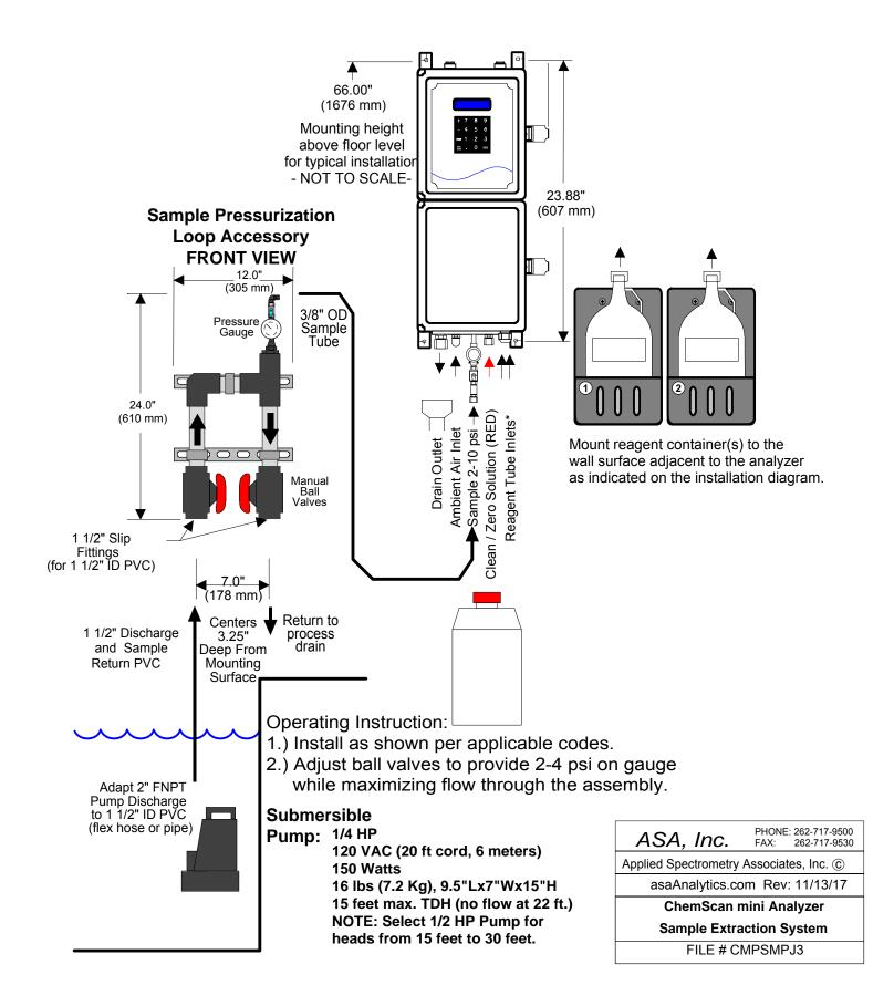
ChemScan mini Analyzer and Sample Extraction Accessory (Sample Pump & Sample Loop)
