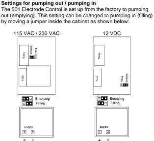
Terminal 13 must always be connected to the high-level electrode. This also applies if you change from pumping out (default) to pumping in. Only here it will function as the STOP electrode.
