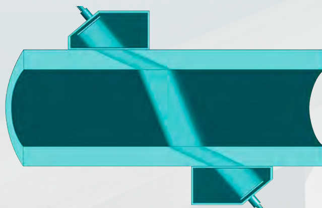
Propagation of ultrasonic shear waves:
