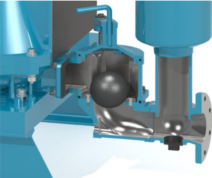
Heavier slurry or sludge at your facility? A ball valve model may help move sewage and sludge more efficiently. Be sure to specify your choice of either ball valve or clack valve at the time of order.
