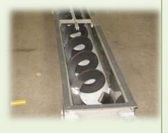
Our shaftless spirals are spun from a heavy, alloy steel bar stock, having up to 250 Brinell hardness. Replaceable UHMWP (Ultra High Molecular Weight Polymer) wear liners line the trough interior protecting it and the spiral from wear. Conveyor troughs, covers, etc. are typically stainless steel for
