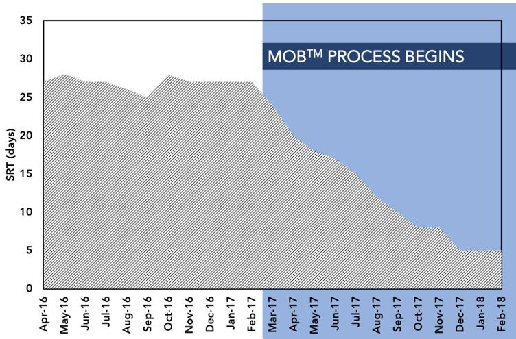
**Figure 8. Monthly average solid retention time (SRT) since April 2016.** The MOB™ process has been able to consistently decrease the SRT from 25 days to 5 days since the installation in March 2017. Kenaf’s high surface area can support concentrated biofilm growth, increasing the treatment capacity by at least 75% within the same reactor configuration.
