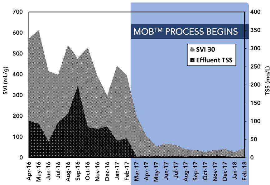
**Figure 10. 30-min Sludge Volume Index (SVI30) and Effluent TSS decreased significantly from an average of 460 mL/g and 90 mg/L to an average of 60 mL/g and 4 mg/L, respectively since March 2017.**
