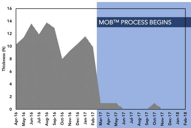
**Figure 9. Sludge blanket thickness in the secondary clarifiers improved from an average of 11 ft to 1 ft as a result of the high settleability of the hybrid matrix.**
