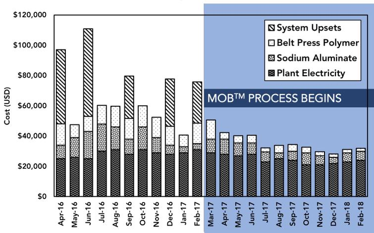
**Figure 7. Monthly cost breakdown** of the Moorefield WWTP since April 2016. The MOB™ Process has decreased the total monthly usage as well as individual usage in electricity, sodium aluminate, and belt press polymer. More importantly, the MOB™ process has eliminated system upsets since the March 2017 installation.
