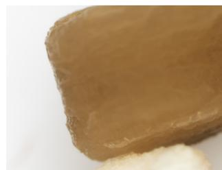
Figure 6. Biofilm growing on a Kenaf particle.
