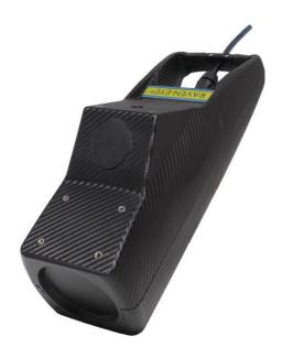
The RAVEN-EYE® is the newest non-contact RADAR area/velocity flow meter for open channel flow measurements from FLOW-TRONIC. The new sensor combines advanced digital Doppler radar velocity sensing technology with most modern and powerful DSP processor technology allowing a patent pending self-learning average velocity calculation. The need for empirical models or time consuming site calibration become obsolete.
