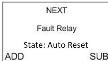
3. Failsafe: Press *ADD* or *SUB* (Yes/No—as indicated on the display screen) to setup Relay 1 as failsafe (or not failsafe). To leave the setting as it is, press *MENU* (Next).
