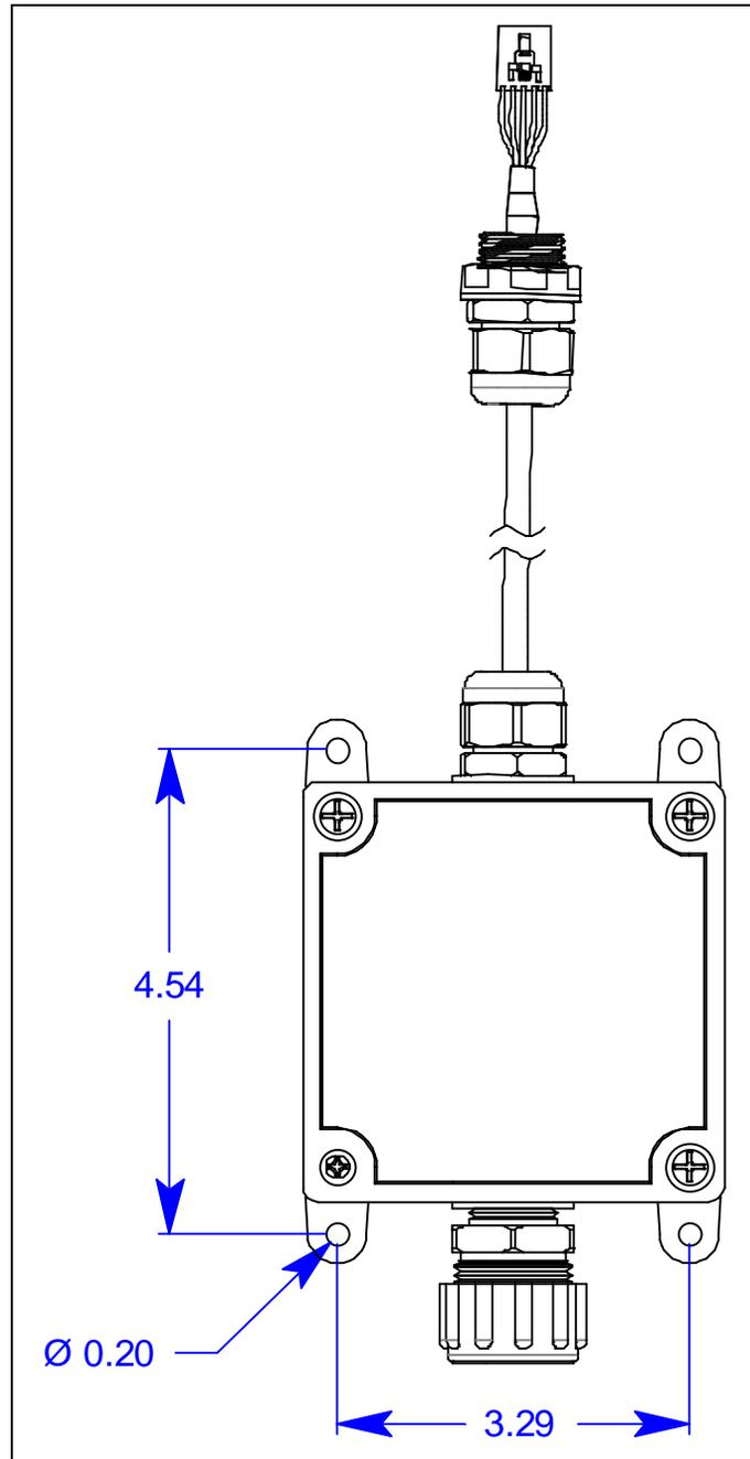
**Figure 5: Remote-Mounted Kit's Detector Junction Box Dimensions**
