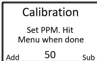
5. Use the ADD and SUB buttons to adjust the concentration match the concentration shown on the calibration cylinder.
