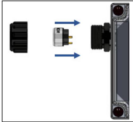
5. Screw the sensor housing cap back onto the sensor housing base, ensuring that the sensor housing cap is only tightened hand tight.
