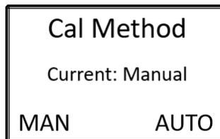
3. Use the ADD button to select manual calibration and the SUB button to select auto calibration.
