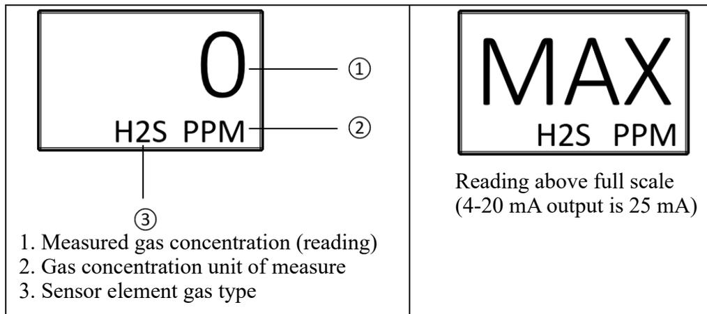
The gas reading is sent back to the controller in 1-minute intervals when the reading is below the background setting (page 28). When the reading surpasses the background setting, the reading is sent back to the controller in 5-second intervals.
