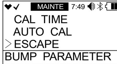
2. Press and release POWER MODE. The instrument returns to the **BUMP PARAMETER** menu.
