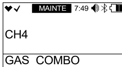
6. Use AIR to change the target gas or turn the channel off.
