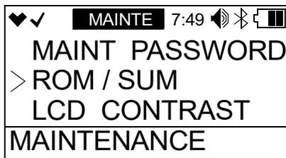
2. Press and release **POWER MODE**. The screen cycles through the main board's ROM/SUM, the sensor board's ROM/SUM, the Bluetooth version, the IR sensor's ROM/SUM (if an IR sensor is installed), and the gas list's ROM/SUM. The ROM is the top value and the SUM is the bottom value.
