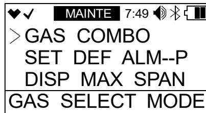
8. **MAINT** at the top of the screen indicates that the GX-3R is in Gas Select Mode.
