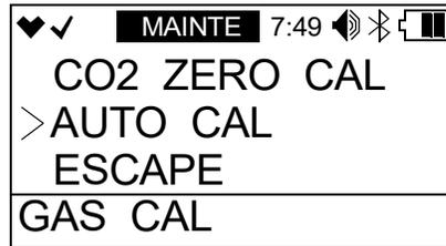
4. Press and release POWER MODE. The Auto Cal screen for gases assigned to Cylinder A displays.
