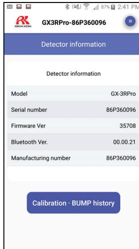
4. To view information for the last successful calibration and bump test, press the “Calibration BUMP history” button.
