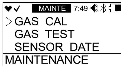
8. **MAINTENANCE** at the top of the screen indicates that the GX-3R is in Maintenance Mode.
