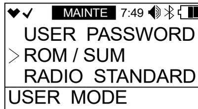
2. Press and release POWER MODE. The screen cycles through the main board's ROM/SUM, the sensor board's ROM/SUM, the IR sensor ROM/SUM (if an IR sensor is installed), and the Bluetooth version. The ROM is the top value and the SUM is the bottom value.
