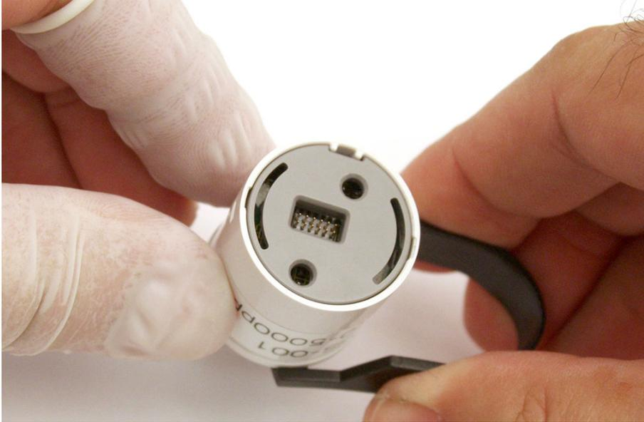
**Figure 25: Using Removal Tool**
