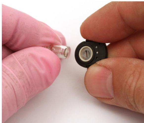
**Figure 28: Reinstalling the Electrode Lamp**
