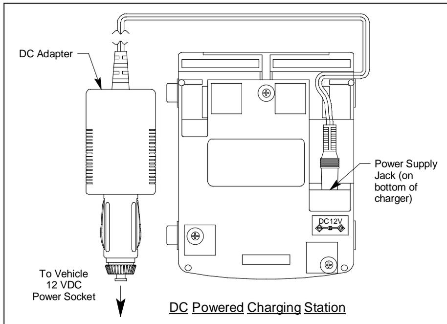
**Figure 19: Connecting the Charging Station's DC Adapter**
