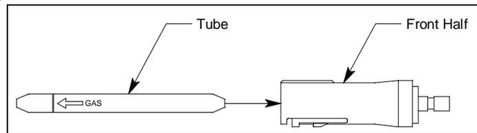
**Figure 38: Inserting New Tube Into Front Half**
