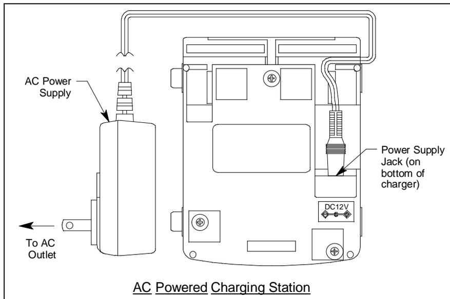
**Figure 15: Connecting the Charging Station's AC Adapter**
