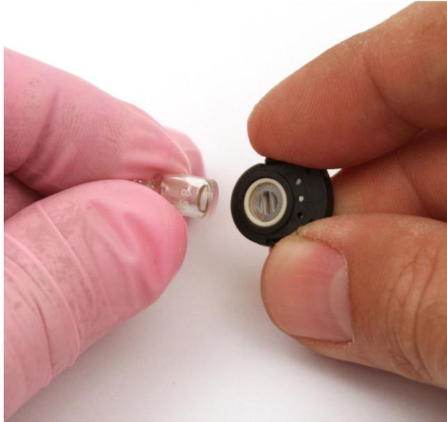
**Figure 31: Reinstalling the Electrode Lamp**
