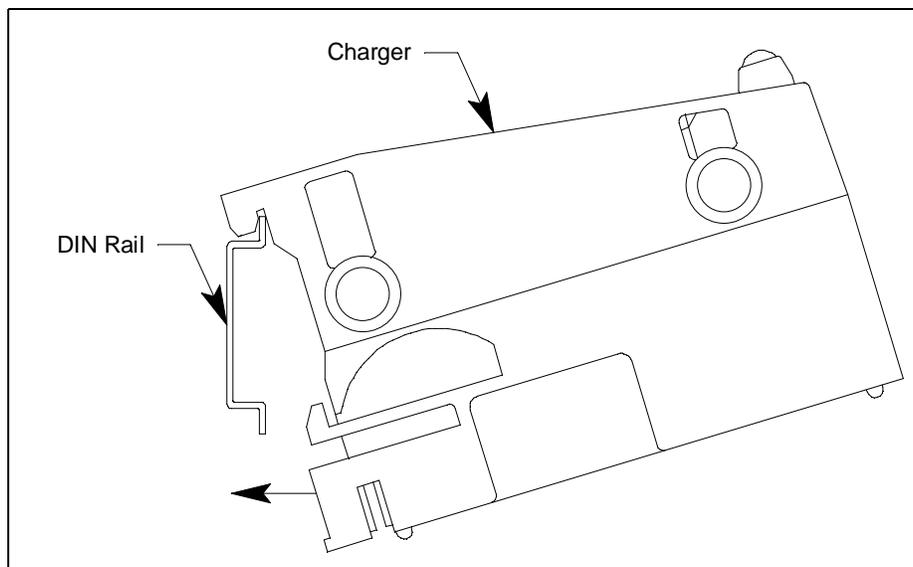
**Figure 5: Installing a Charger on the DIN Rail**
