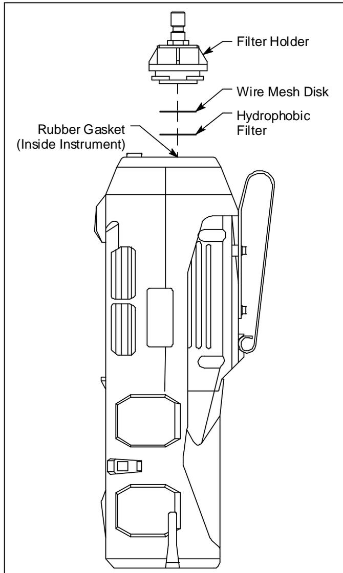
**Figure 24: Changing the Filter & Wire Mesh Disk**
