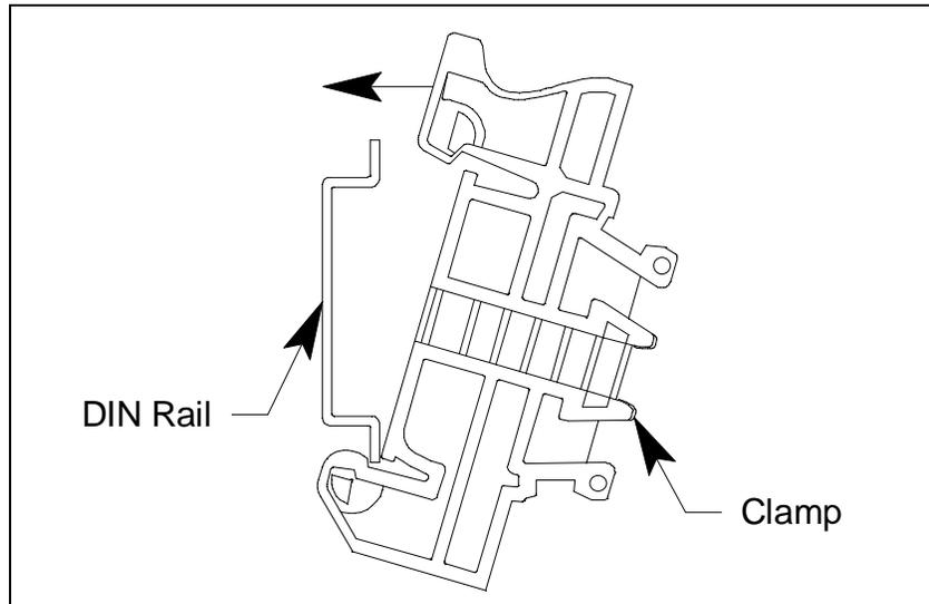
**Figure 6: Clamp Installation**
