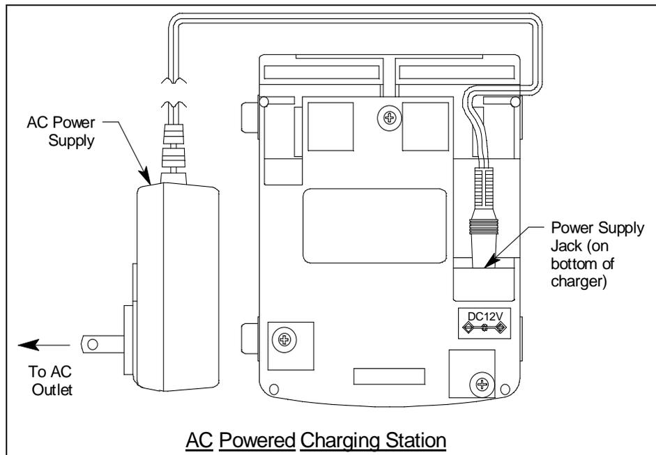
**Figure 18: Connecting the Charging Station's AC Adapter**
