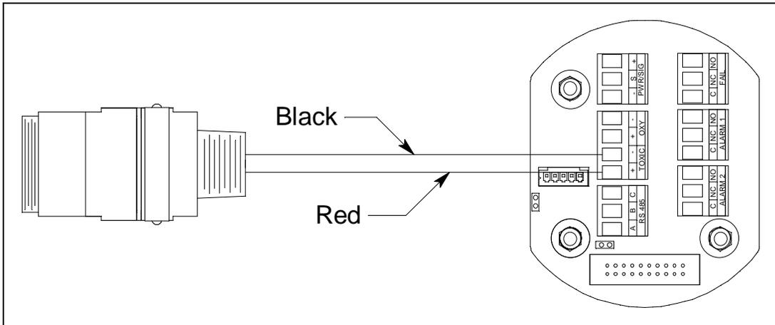
**Figure 26: H<sub>2</sub>S/CO Detector Wiring, CSA**
