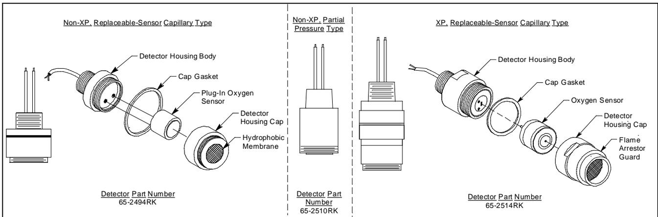
**Figure 4: Oxygen Detectors**
