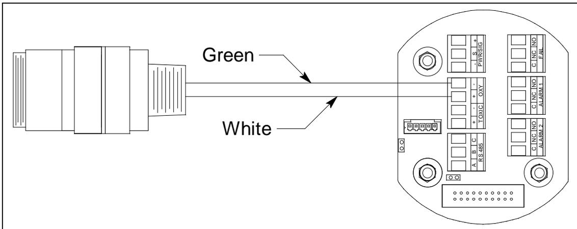
**Figure 24: CSA Capillary Type Oxygen Detector Wiring**
