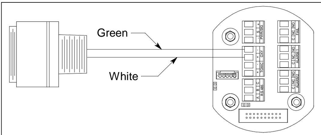
**Figure 25: Capillary Type Replaceable Sensor Oxygen Detector Wiring**
