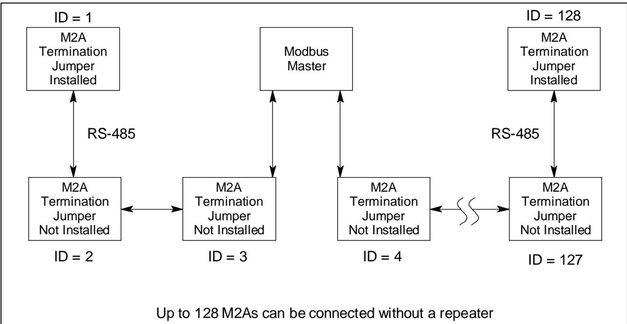
**Figure 35: Multiple M2As in a Two Branch Configuration**
