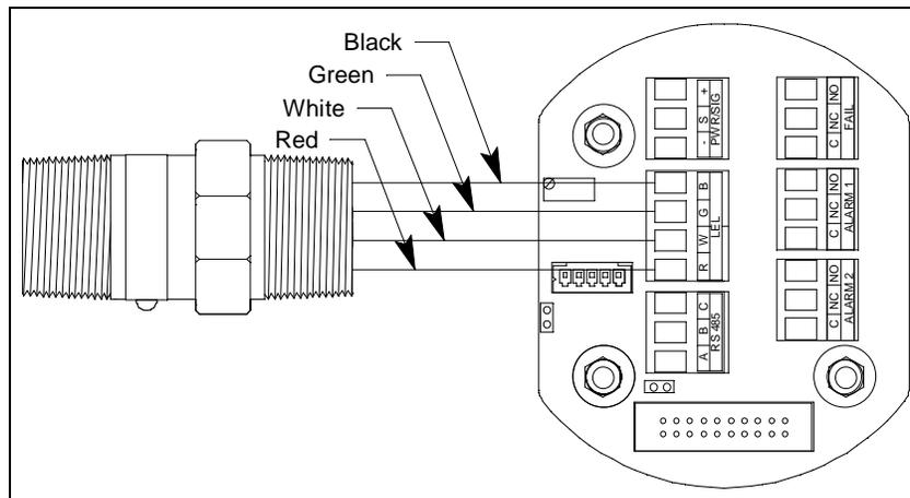
Figure 22: IR Combustible/IR CO<sub>2</sub> Detector Wiring
