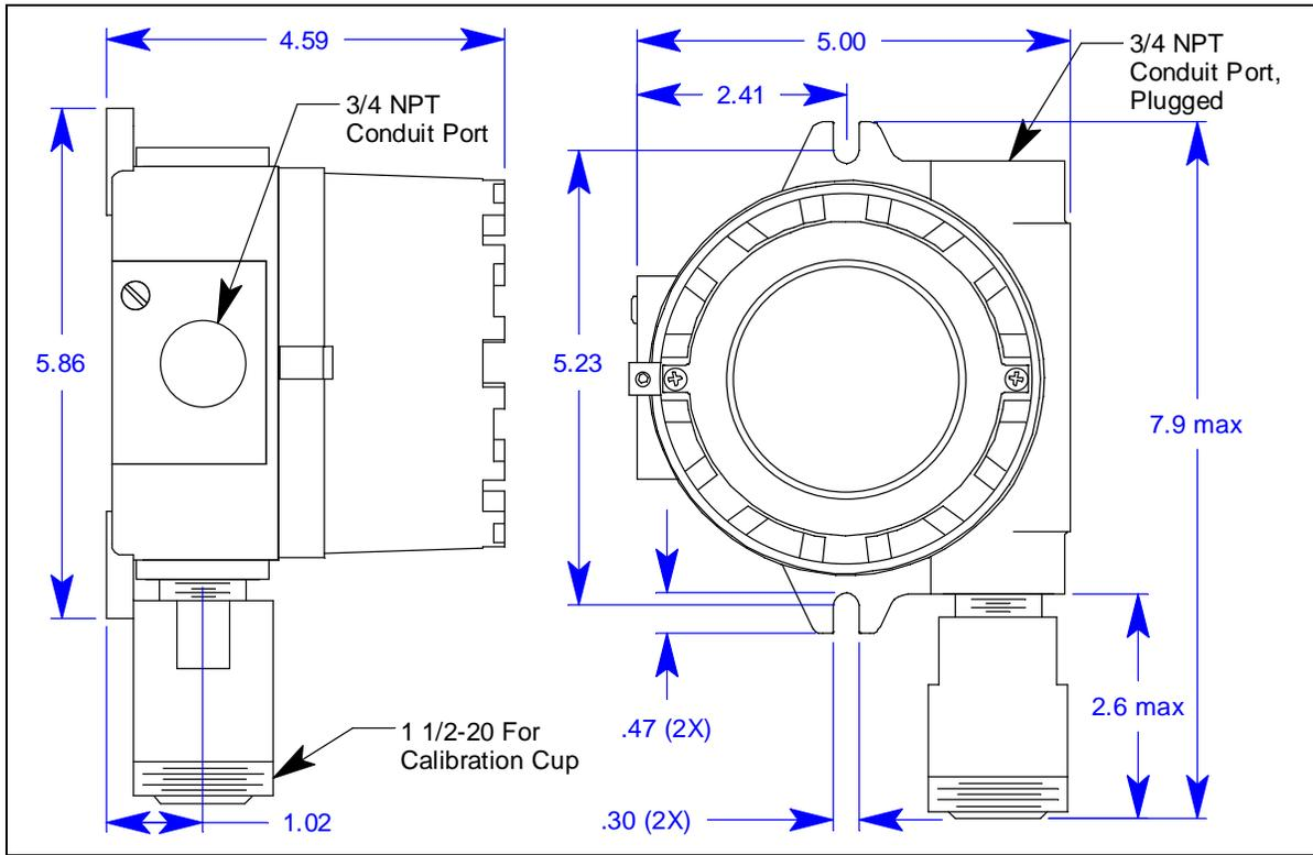
**Figure 16: Outline & Mounting Dimensions, Oxygen, Partial Pressure Type**
