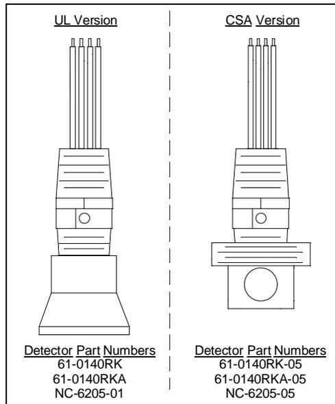
**Figure 2: Catalytic Sensors**
