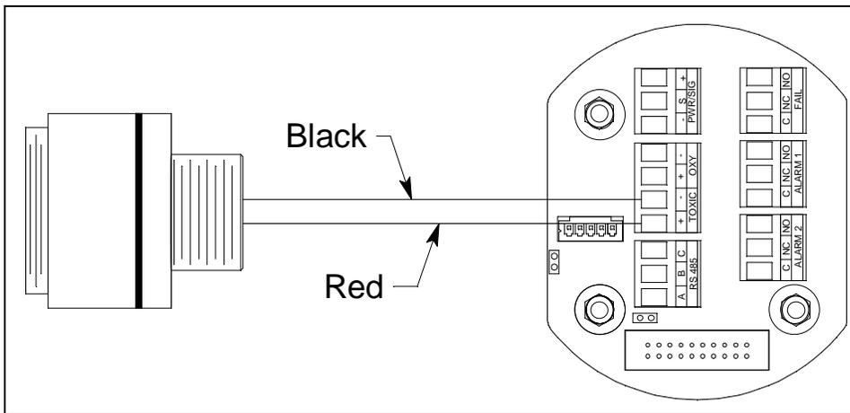
**Figure 27: H<sub>2</sub>S/CO Detector Wiring**
