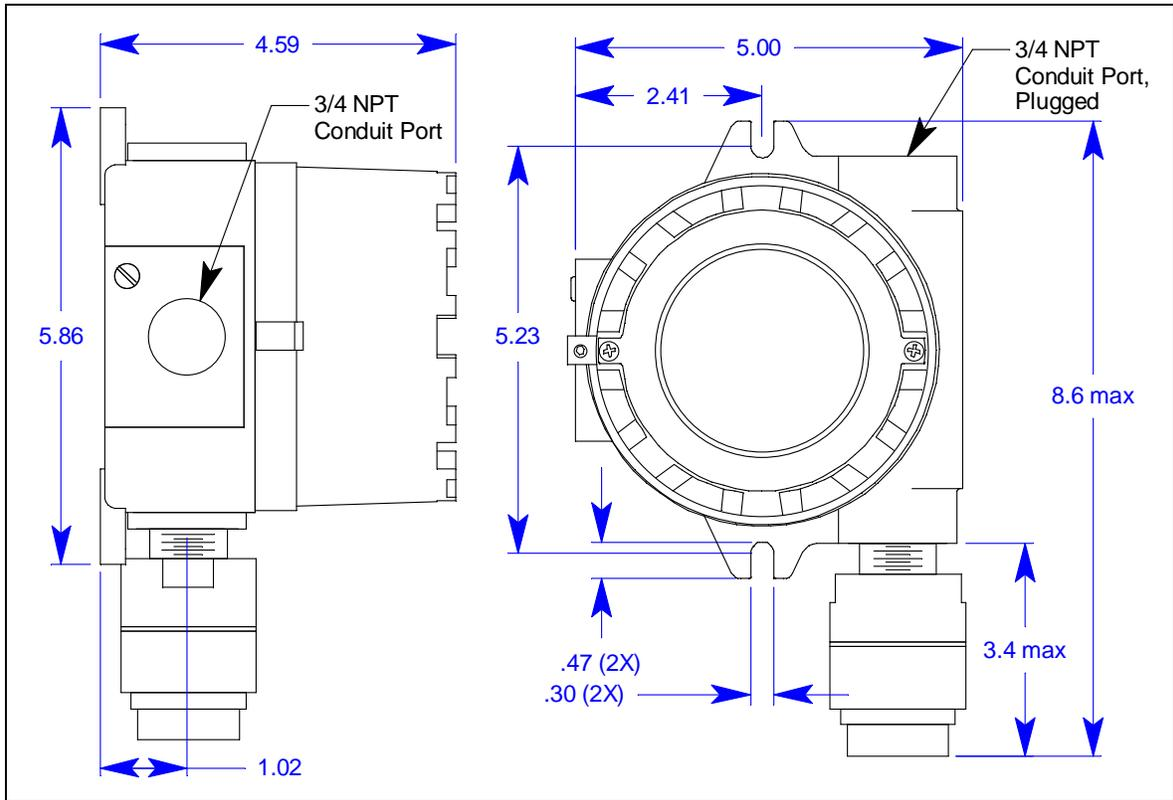
Figure 18: Outline & Mounting Dimensions, H<sub>2</sub>S, CO, and Oxygen, CSA, Explosion-Proof
