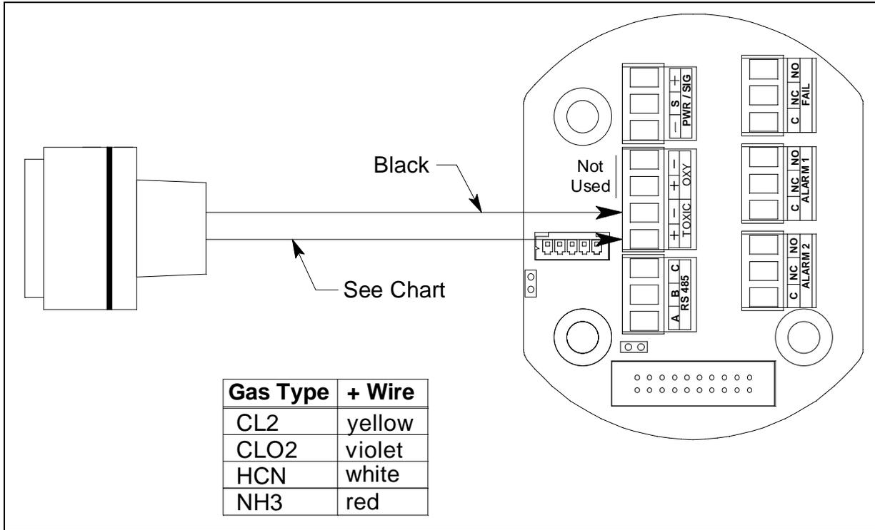
**Figure 29: CT-7 Series Toxic Detector Wiring**
