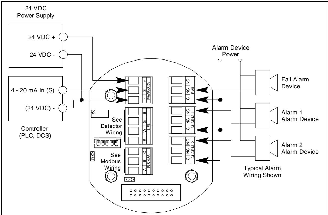
**Figure 36: PLC and DCS Device Wiring**
