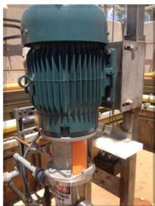
The series 35FP utilizes a close coupled rugged and reliable U.S.A. manufactured BALDOR TEFC severe duty motor for indoor or outdoor service in corrosive environments. The motor is bolted to a Magnaloy cast aluminum motor mount assembly for shaft alignment and easy access to the shaft coupling.
